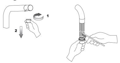
It is recommended that you periodically clean the aerator of your faucet. To do so, unscrew the aerator holder from its own seat. Simply using a toothbrush, or something similar, rub the filter under the water, removing the impurities and any build up. Screw the areator back into place.
